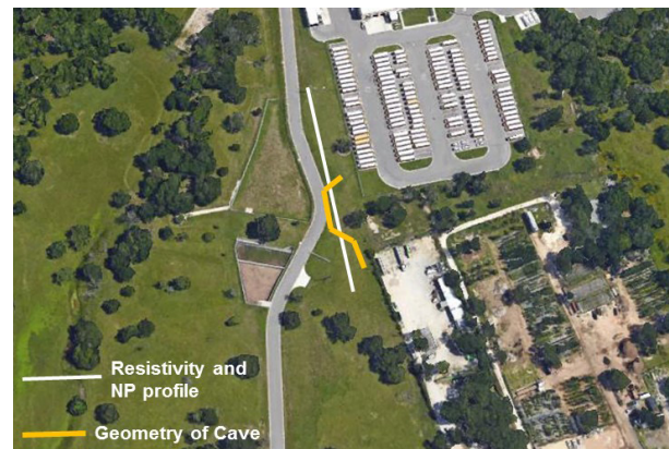
Figure 15. Site map showing the location of the geophysical profile, and the geometry of the cave, which was defined by trenching. The length of the geophysical profile is about 122 meter (400 feet).
